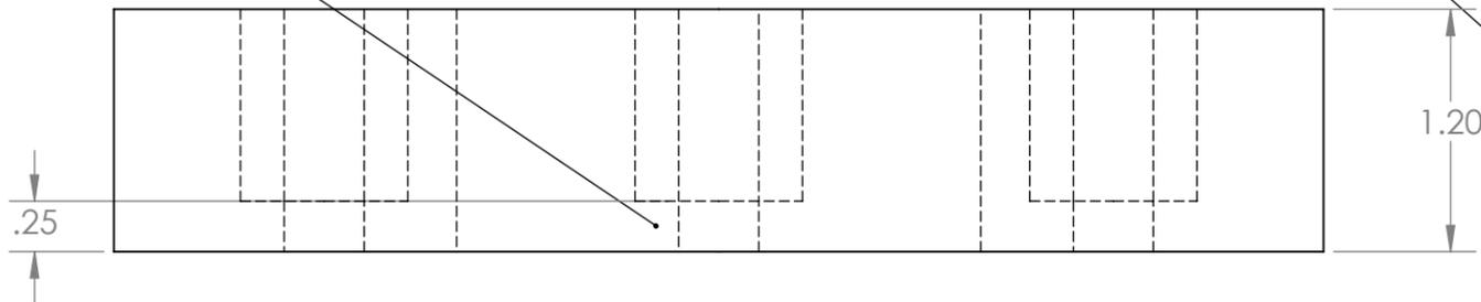
New bolts to attach spacer + coil assembly to coil bucket.
